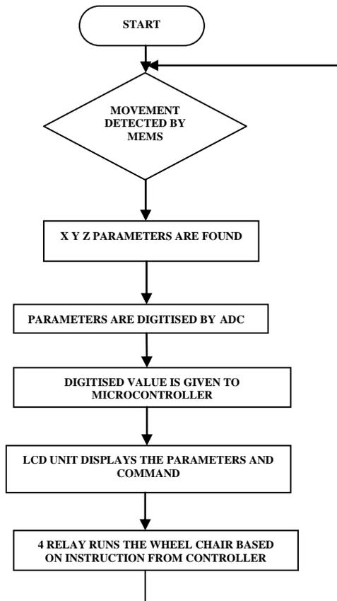
Figure 2: Flow chart for working of mems
