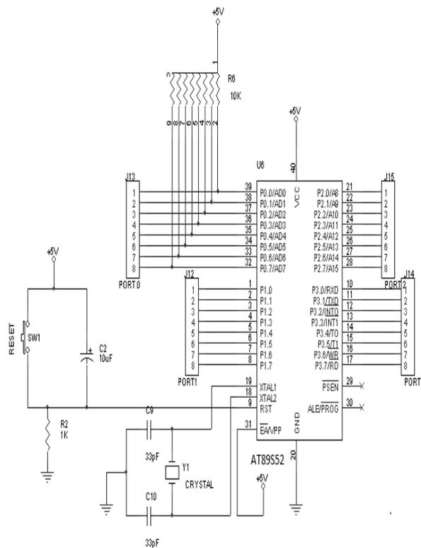
Figure 4: AT89S52 Controller circuit
