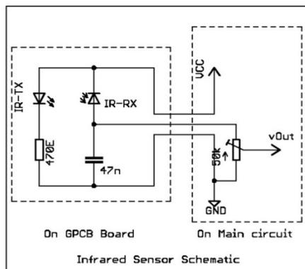
Figure 13: Circuit diagram of IR sensor
