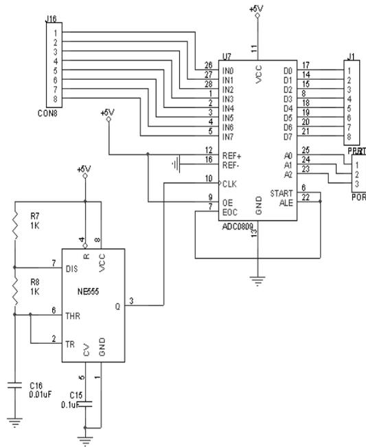
**Figure 5: ADC0809 circuit diagram**
