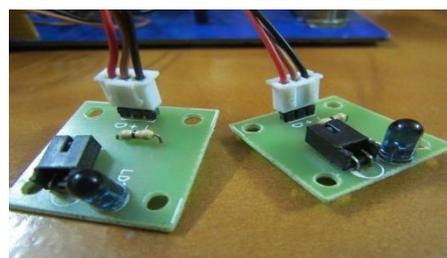
**Figure 16: Two IR sensors**
