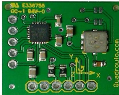
Figure 9(a) Gyroscope IC
