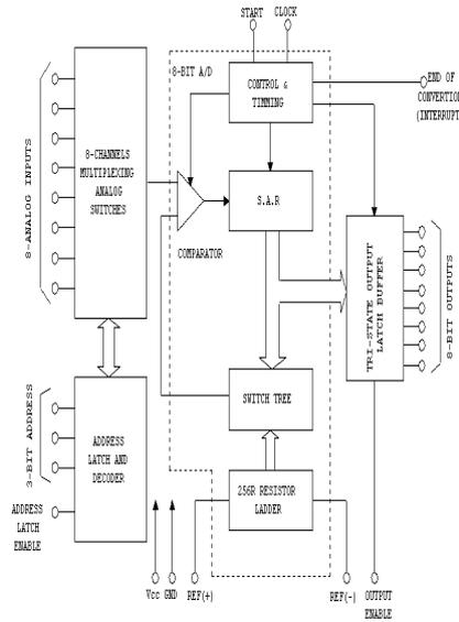
Figure 8: Block diagram of ADC 0809
