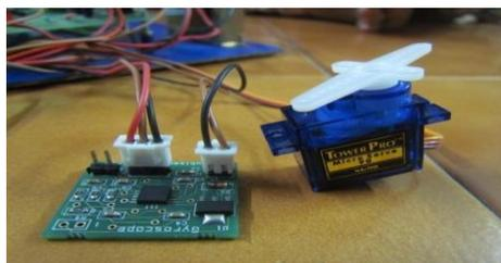
**Figure 19: Gyroscope and servomotor**
