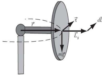
Figure 10 (b) A simple gyroscope, showing precession
