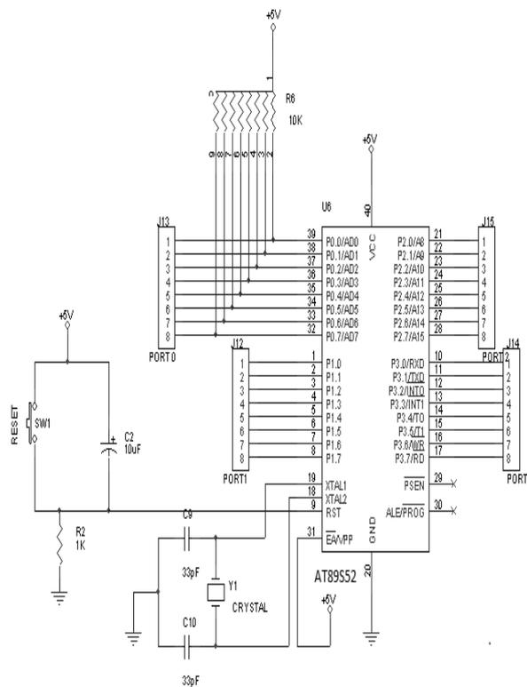
Figure 4: AT89S52 Controller circuit
