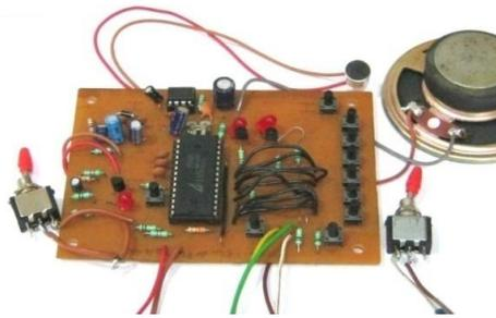
**Figure 14: Voice board APR9600 circuit**
