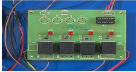
**Figure 20: Four relay board**
